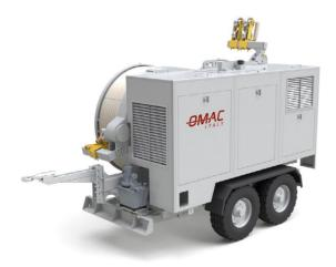
Hydraulic machine designed to operate both as a tensioner and as puller, fit to string one or two ropes or conductors. Two hydraulic circuits allow to tension at constant force even varying the speed of stringing. The two circuits can be used independently or simultaneously, with automatic forces partition. In puller mode, 2 closed hydraulic circuits allow to vary the speed in both directions, allowing to
