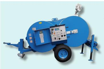
Hydraulic machine designed to operate both as a tensioner and as puller, fit to string one or two ropes or conductors. One hydraulic circuit allows to tension at constant force even varying the speed of stringing. In puller mode, one hydraulic circuit allows to continuously vary the speed in both directions.
