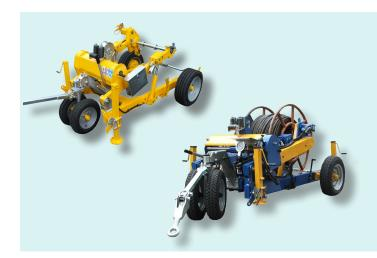
Reel-winder trolley fit for reel transport and wire recovering/releasing, designed to be used with pullers, puller-tensioners or hydraulic power units, from which it receives the transmission needed to move the reel. It can even be fitted with own motorization.
