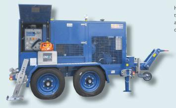
Hydraulic puller fit to pull one rope in laying underground transmission cables and optics fibre cables. One hydraulic circuit allows to continuously vary the speed in both directions by operating one control device.
