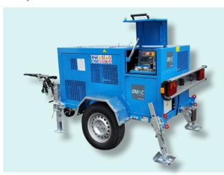
Hydraulic puller fit to pull one rope in laying underground transmission cables and optics fibre cables. One hydraulic circuit allows to continuously vary the speed in both directions by operating one control device.
