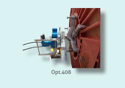
Stands fit for steel or wooden reels, used for lifting a reel and braking it while stringing the conductor/cable. The reel stands, as an option, can be hydraulically driven by a hydraulic power unit. Reel-stands are supplied in pairs.
