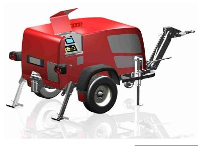
Hydraulic puller fit to pull one rope in laying underground power and optics fibre cables. One hydraulic circuit allows to continuously vary the speed in both directions.
