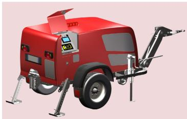
Hydraulic puller fit to pull one rope in laying underground power and optics fibre cables. One hydraulic circuit allows to continuously vary the speed in both directions.
