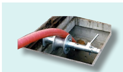
Adjustable boom with aluminium cable roller.
