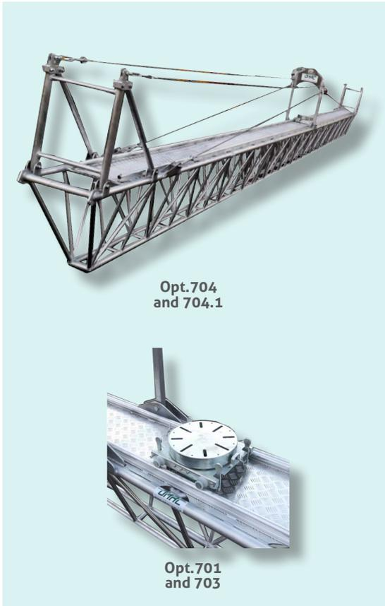
Suspension platform for overhead line works. Aluminium alloy structure. Made of two or more trapezoidal sections, with central fitting and lateral hooks for anchoring. Complete with wire ropes and turnbuckles.
