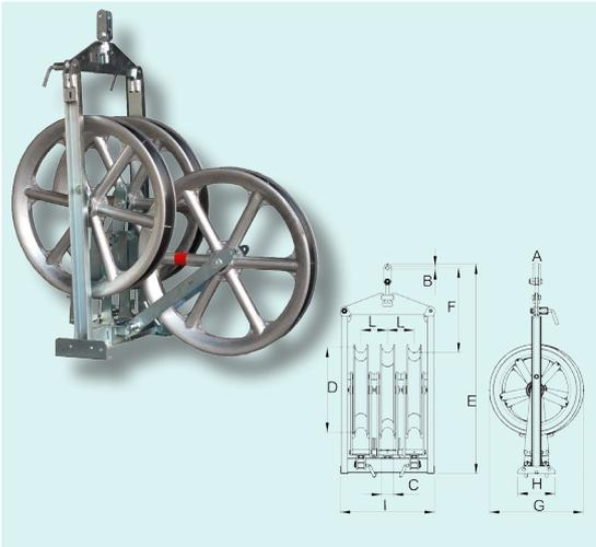
Detachable three-sheave running out block fit for stringing two- three-bundled conductors. The frame contains 3 running-out blocks that can be used singularly. Aluminium sheaves mounted on sealed ball bearings. Grooves lined with nylon sectors. Galvanised steel frame. Central sheave mounted on double bearings. Demountable attachment revolving by 90°.
