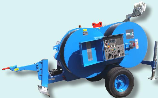
Hydraulic machine designed to operate both as a tensioner and as puller, fit to string one or two ropes or conductors. One hydraulic circuit allows to tension at constant force even varying the speed of stringing. In puller mode, one hydraulic circuit allows to continuously vary the speed in both directions.
