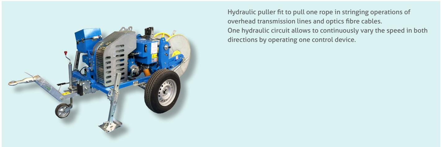
Hydraulic puller fit to pull one rope in stringing operations of overhead transmission lines and optics fibre cables. One hydraulic circuit allows to continuously vary the speed in both directions by operating one control device.
