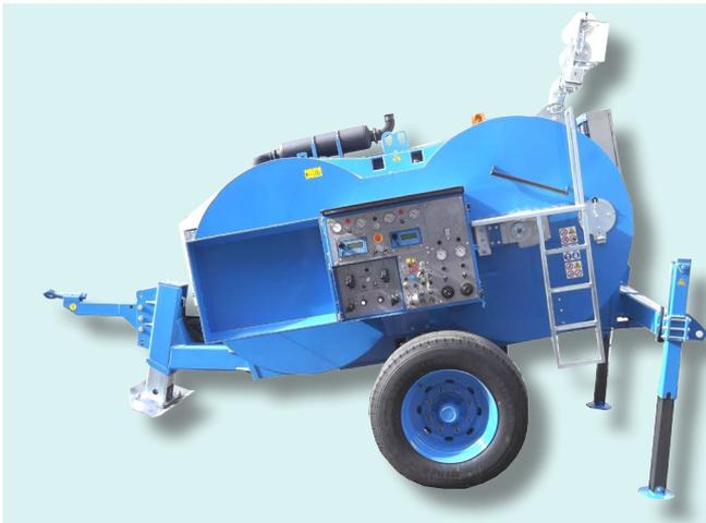
Hydraulic machine designed to operate both as a tensioner and as puller, fit to string one or two ropes or conductors. Two hydraulic circuits allow to tension at constant force even varying the speed of stringing. The two circuits can be used independently or simultaneously, with automatic forces partition. In puller mode, 2 closed hydraulic circuits allow to vary the speed in both directions, allowing to use one of the hydraulic circuits or both of them matched.
