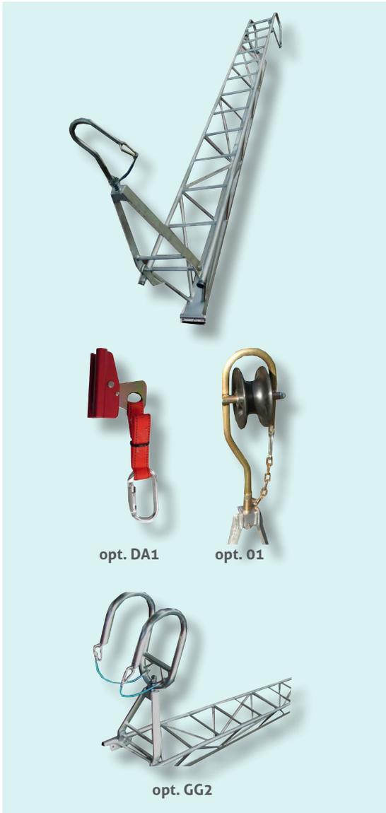
Anchoring ladder made of light aluminum alloy, with steps made of antislipping material and suspension hooks in hot-dip galvanized steel. The ladder is complete with a fix hook for tower, 220mm opening, and a swivel hook for leaning on the conductor, to use the ladder in horizontal position. The ladders have trapezoidal shape.
