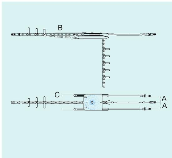
**F153.2 Balanced type** running board for 2-bundle conductors, fit for connecting the pulling rope to 2 conductors.
