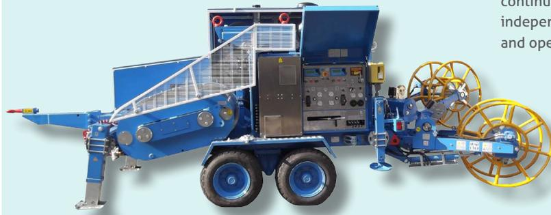
Hydraulic puller fit to pull one or two ropes in stringing operations of overhead transmission lines. Two hydraulic circuits allow to continuously vary the speed in both directions by operating two independent control devices. The two circuits may also be matched and operated together by one control device.
