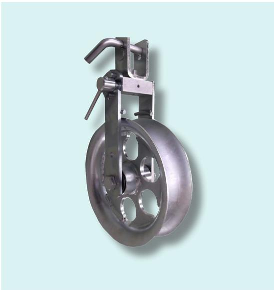
Running out block fit for stringing shield wires. Galvanized steel sheave mounted on ball bearings. Galvanized steel frame with non-fleeting device.
