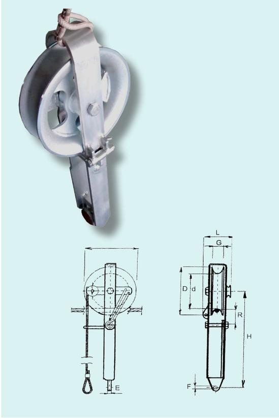
Counter-pull running-out block. Galvanised steel frame, openable side, with swivelling hooks on the ends. Automatic releasing device for recovering the unit.
