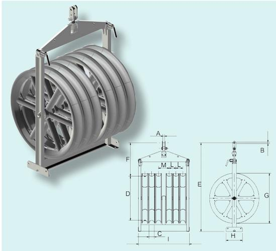
Six-sheave running out block, fit for stringing 6 conductors. Aluminium sheaves mounted on sealed ball bearings. Grooves lined with nylon sectors. Steel frame with non-fleeting devices on lateral sheaves. Demountable attachment revolving by 90°.
