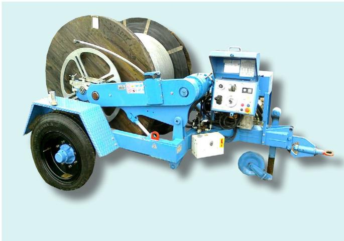
Trailer for reels, fit for recovering and releasing ropes and conductors to/from wooden or steel reels. The reel, operated by a hydraulic motor, allows to recover the wire or conductor (puller use) and to release it (tensioner use).
