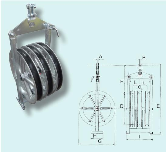
Three-sheave running out block fit for stringing two- three-bundled conductors. Aluminium sheaves mounted on sealed ball bearings. Grooves lined with nylon sectors. Galvanised steel frame with non-fleeting devices on lateral sheaves. Demountable attachment revolving by 90° (available with tight wheel).
