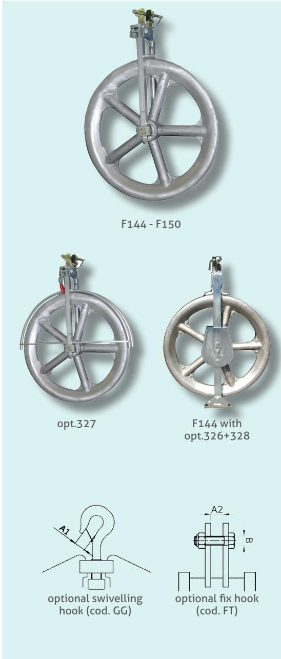
Single sheave running out block fit for stringing one conductor. Aluminium sheave mounted on sealed ball bearings. Groove lined with nylon sectors. Openable galvanised steel frame with non-fleeting device. Standard swivelling fork attachment.
