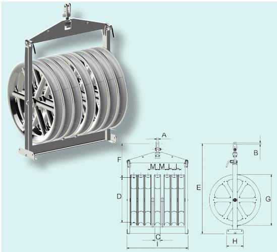
Seven-sheave running out block, fit for stringing 4 or 6 conductors. Aluminium sheaves mounted on sealed ball bearings. Grooves lined with nylon sectors. Steel frame with non-fleeting devices on lateral sheaves. Demountable attachment revolving by 90°.
