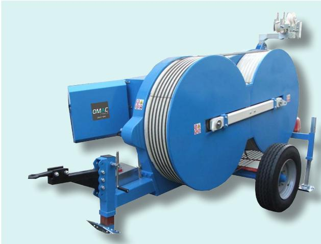
Hydraulic tensioner fit to string one or two conductors or optical fiber cables. One hydraulic circuit allows to tension at constant force even varying the speed of stringing. Equipped with engine for pull-back performances.
