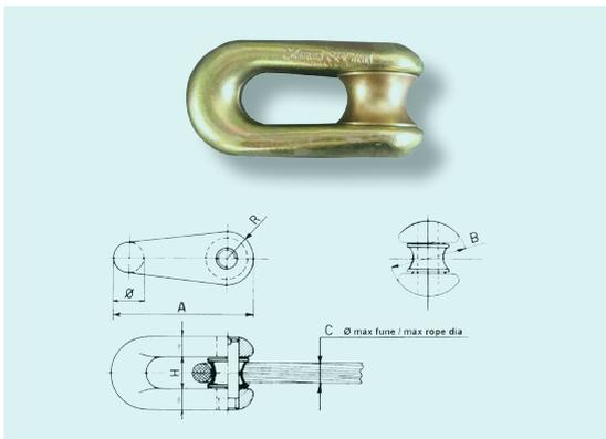
Joint made of high tensile galvanised steel, fit to connect pilot rope lengths and pulling rope. Designed to pass on the capstan grooves of pullers or puller/tensioners.
