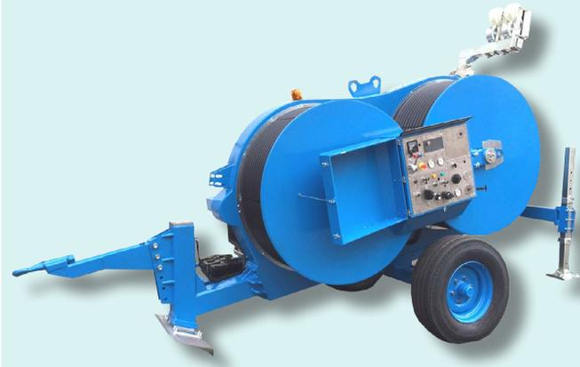
Hydraulic machine designed to operate both as a tensioner and as a puller, fit to string one or two ropes or conductors. One hydraulic circuit allows to tension at constant force even varying the speed of stringing. In puller mode, one hydraulic circuit allows to continuously vary the speed in both directions.
