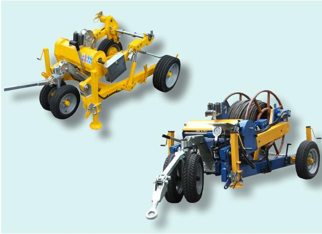
Reel-winder trolley fit for reel transport and wire recovering/releasing, designed to be used with pullers, puller-tensioners or hydraulic power units, from which it receives the transmission needed to move the reel. It can even be fitted with own motorization.
