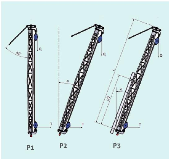
Gin poles made of aluminium alloy tubular structure welded with TIG system.
