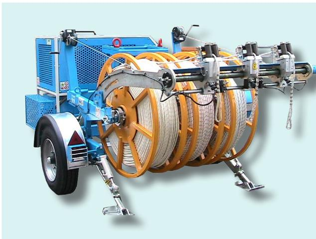
Trailer designed for transporting reels as well as for recovering and releasing ropes and conductors to/from wooden or steel reels. The trailer can host up to 3 or 4 reels. The reels, operated by a hydraulic motor, allow to recover the wires (like a puller) and to release them (braked tension).
