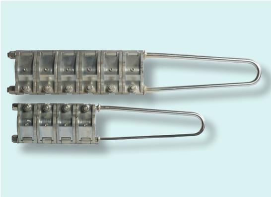
Multi-unit come-along clamp fit for pulling and anchoring overhead conductors and steel wire ropes. Made of steel elements, with aluminium liners for conductors.
