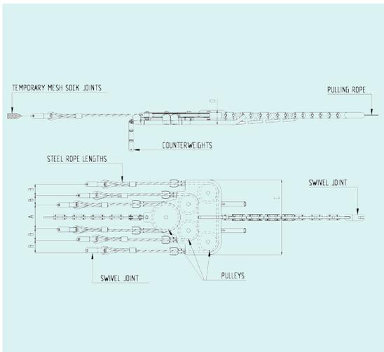
**Balanced type** running board for 6-bundle conductors fit for connecting the pulling rope to 6 conductors.
