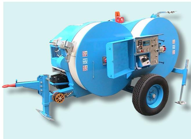
Hydraulic tensioner fit to string one conductor or fiber optic cable. One hydraulic circuit allows to tension at constant force even varying the speed of stringing. Equipped with engine for pull-back performances.
