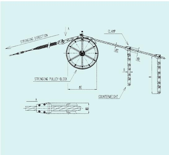
Antitwisting counterweight fit for stringing overhead fiber optics cables (OPGW).
