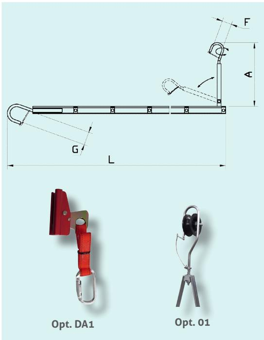
Suspension ladder fit for vertical or horizontal use. Aluminum alloy structure welded with TIG system, complete with T profile for anti-fall device. Interchangeable tower hook made of galvanized steel. The foldable end with conductor hook allows to use the ladder as a horizontal platform. also available versione C167.F...S, working load 200 daN.
