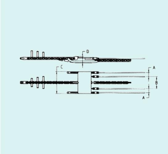
**Fixed type** running board for 4-bundle conductors fit for connecting the pulling rope to 4 conductors. The running board is made up of:
