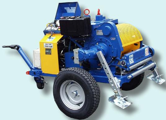
Hydraulic winch fit to pull one rope in service operations such as setting-ups and adjustment of transmission lines and underground cables laying. Direct pull on the drum. One closed hydraulic circuit allows to continuously vary the speed in both directions by operating one control device.
