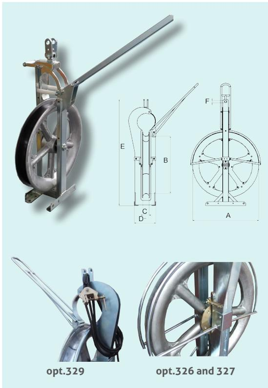
Single sheave block fit for stringing a pilot rope by helicopter. Proper devices allow to position the pulling rope in the sheave groove and keep it inside the groove during stringing operations. Aluminium sheave mounted on waterproof bearings. Groove lined with nylon sectors. Galvanized steel frame. Fix attachment.
