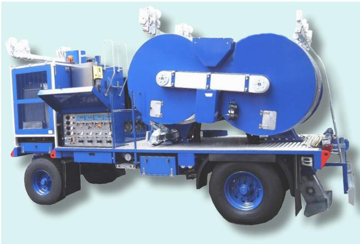
Hydraulic machine designed to operate both as a tensioner and as puller, fit to string 1, 2, 3 or 4 ropes or conductors. Four hydraulic circuits allow to tension at constant force even varying the speed of stringing. The four circuits can be used independently or simultaneously, with automatic forces partition. In puller mode, four closed hydraulic circuits allow to vary the speed in both directions, allowing to use one of the hydraulic circuits or all of them matched.
