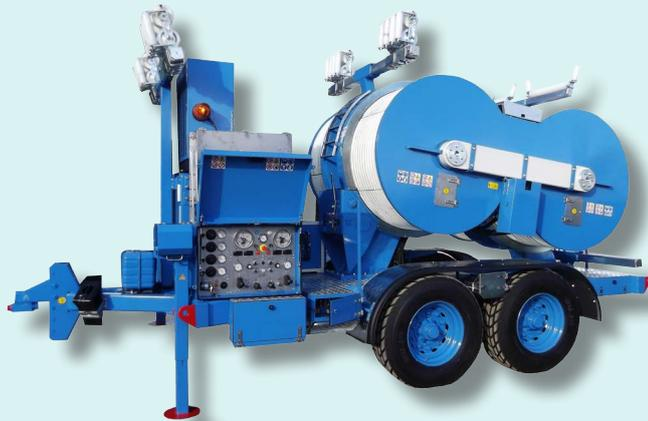
Hydraulic tensioner fit to string 1, 2, 3 or 4 (up to 6 on demand) conductors. Two hydraulic circuits allow to tension at constant force even varying the speed of stringing. The two circuits can be used independently or simultaneously, with automatic forces partition. Equipped with engine for pull-back performances. In pull-back mode, two hydraulic circuit allow to vary the speed in both directions, allowing to use one of the hydraulic circuits or both of them matched.
