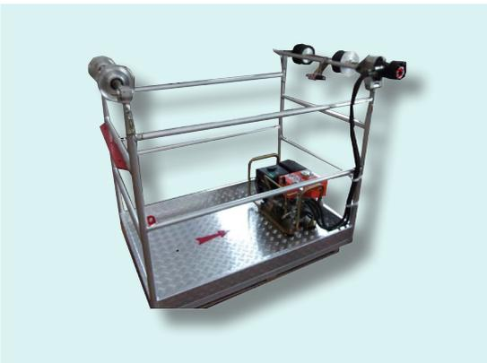
Motorized line-car for 2 linemen, fit for 2-, 3- or 4-bundle conductor lines.
