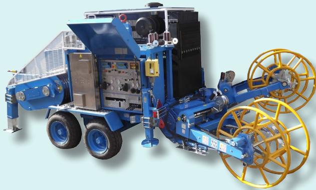
Hydraulic puller fit to pull one or two ropes in stringing operations of overhead transmission lines. Two hydraulic circuits allow to continuously vary the speed in both directions by operating two independent control devices. The two circuits may also be matched and operated together by one control device.
