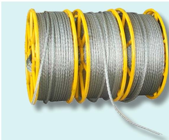
Anti-twisting galvanised steel rope specifically designed for stringing operations. Made up of 12 braided strands. High resistant to break, antitwisting, flexible, safe and easy to handle. The linear contact between the braided strands grants a low stress on the rope. Supplied wound up on steel or wooden reels.
