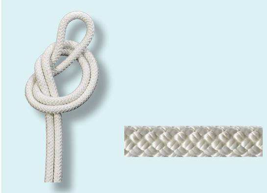
Pilot rope made of an external polyester mesh stocking and a hi-tenacity nylon core. Double torsion. Highly resistant to wear and UV rays. white colour. Supplied wound up on wooden reels or in coils.
