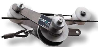
Braking device for cradle blocks. Positioned behind the cradles, to keep the distance between the cradles. Aluminium frame and aluminium, rubber wheels mounted on ball-bearings.
