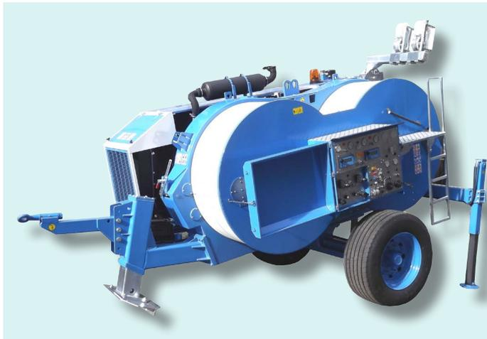
Hydraulic tensioner fit to string one or two conductors. Two hydraulic circuits allow to tension at constant force even varying the speed of stringing. The two circuits can be used independently or simultaneously, with automatic forces partition. Equipped with engine for pull-back performances. In pull-back mode, two hydraulic circuit allow to continuously vary the speed in both directions, allowing to use one of the hydraulic circuits or both of them matched.
