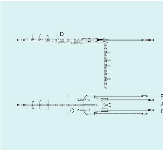
**Balanced type** running board for 4-bundle conductors fit for connecting the pulling rope to 4 conductors.
