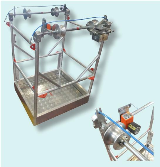
Line-car for twin conductor lines (2 cond.). Made of light alloy structure with nylon wheels mounted on ball-bearings. Stationary brake and metercounter. Also available for 3-bundle lines (3 conductors): mod. **C155.A.3**
