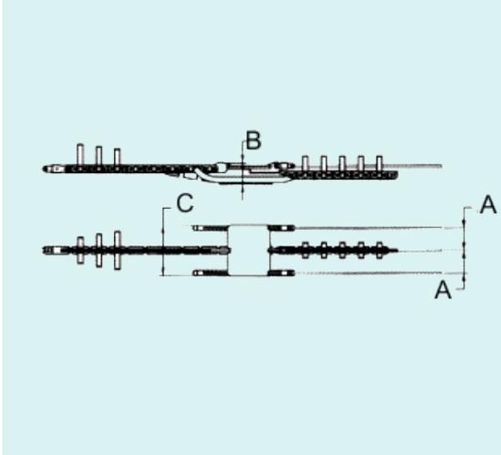
**F153.2...F Fixed type** running board for 2-bundle conductor, fit for connecting the pulling rope to 2 conductors. The running board is made up of:
