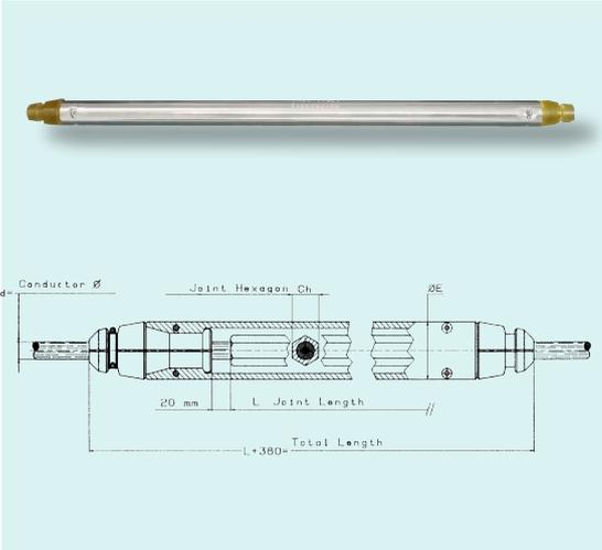
Joint protector made up of two galvanised steel shells. The ends are shaped to host the rubber protections. It is fit to limit the bending radius of the conductor during the passage in the running out blocks.
