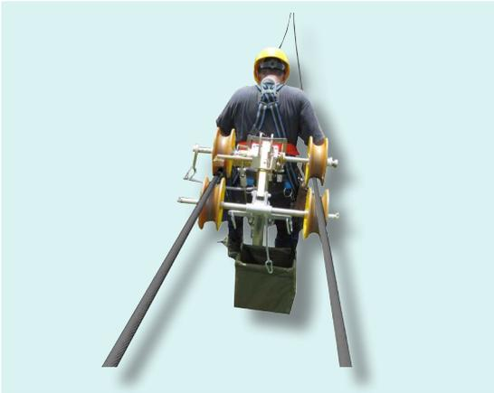
Bicycle for single, twin, 3- and 4-bundle conductor lines.
