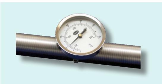
Thermometer for conductors. The dial diameter 80 mm, with incorporated sensor, can be fixed easily on the conductor by means of its elastic clamp.
