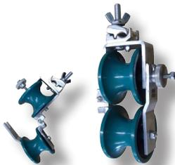
Cradle block designed for the replacing existing cables, with clamp for ropes diameter from 10 to 20 mm. Two nylon wheels and aluminium frame.
