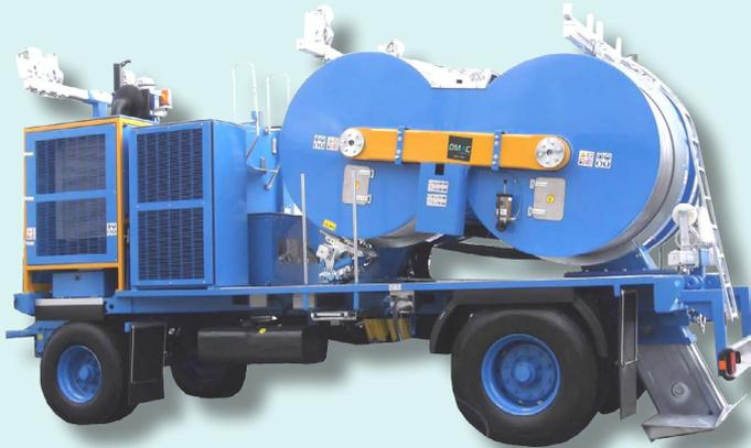
Hydraulic machine designed to operate both as a tensioner and as a puller, fit to string 1, 2, 3 or 4 ropes or conductors. Two hydraulic circuits allow to tension at constant force even varying the speed of stringing. The two circuits can be used independently or simultaneously, with automatic forces partition. In puller mode, 2 closed hydraulic circuits allow to vary the speed in both directions, allowing to use one of the hydraulic circuits or both of them matched.
