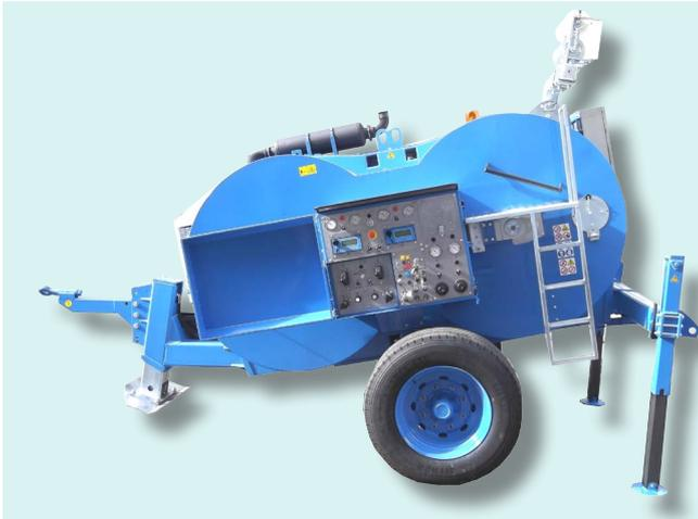
Hydraulic machine designed to operate both as a tensioner and as a puller, fit to string one or two ropes or conductors. Two hydraulic circuits let to tension at constant force even varying the speed of stringing. The two circuits can be used independently or simultaneously, with automatic forces partition. In puller mode, 2 closed hydraulic circuits allow to vary the speed in both directions, allowing to use one of the hydraulic circuits or both of them matched.
