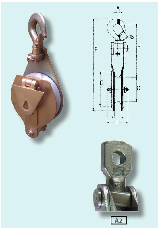
Openable snatch block. Aluminium sheave mounted on ball bearings. Aluminium frame with openable side. Standard steel hook attachment.
