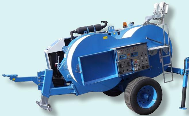
Hydraulic tensioner fit to string one or two conductors. Two hydraulic circuits allow to tension at constant force even varying the speed of stringing. The two circuits can be used independently or simultaneously, with automatic forces partition. Equipped with engine for pull-back performances. In pull-back mode, two hydraulic circuit allow to continuously vary the speed in both directions, allowing to use one of the hydraulic circuits or both of them matched.
