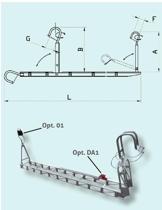
Suspension ladder fit for vertical and horizontal use. Aluminum alloy structure welded with TIG system, complete with T profile for anti-fall device. The two foldable ends, fitted with hooks for tower and for conductor, allow to use the ladder as a horizontal platform. also available versione C167.G...S, working load 200 daN.
