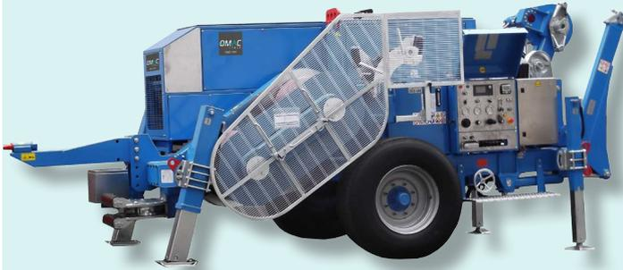
Hydraulic puller fit to pull one rope in stringing operations of overhead transmission lines. One hydraulic circuit allows to continuously vary the speed in both directions by operating one control device.
