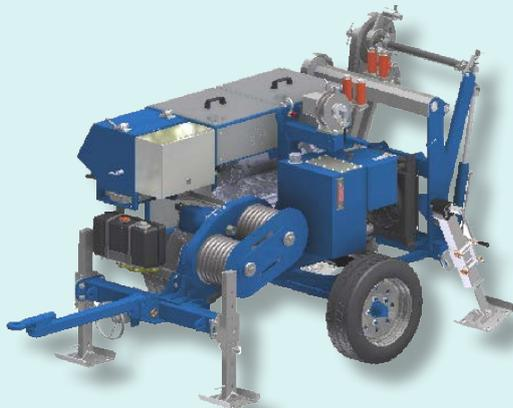
Hydraulic puller fit to pull one rope in stringing operations of overhead transmission lines. One hydraulic circuit allows to continuously vary the speed in both directions by operating one control device.
