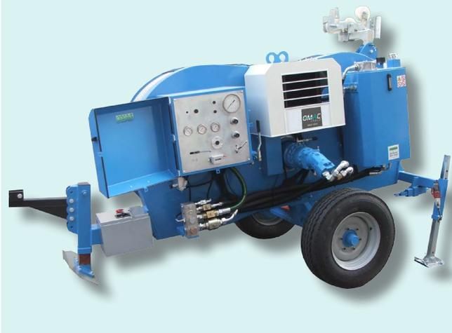
Hydraulic tensioner fit to tension one conductor or fiber optic cable. One hydraulic circuit allows to tension at constant force even varying the speed of stringing.
