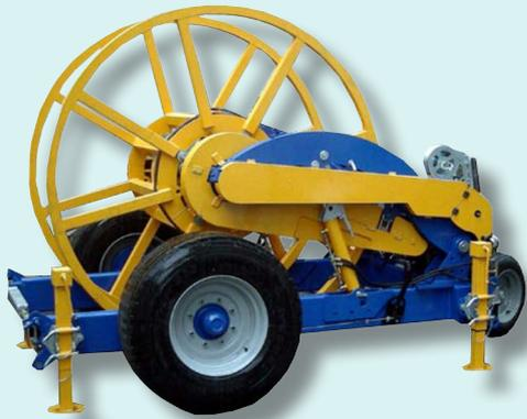
Reel-winder trolley designed for recovering/pulling and releasing ropes and conductors to/from steel reels. The reel is operated by a hydraulic motor fed by a separate power unit or by the auxiliary hydraulic circuit of a puller, tensioner or puller/tensioner.
