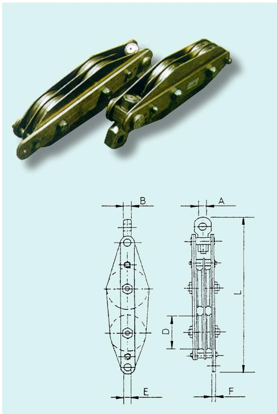
Tackle block for high voltage lines. Steel frame with 4 or 6 steel sheaves mounted on waterproofed ball bearings. Supplied in pairs.
