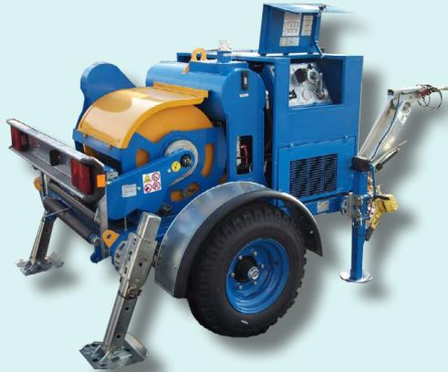
Hydraulic winch fit to pull one rope in service operations such as setting-ups and adjustment of transmission lines and underground cables laying. Direct pull on the drum. One closed hydraulic circuit allows to continuously vary the speed in both directions by operating one control device.
