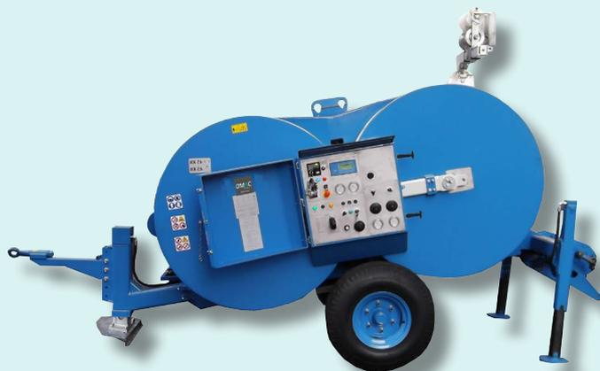
Hydraulic machine designed to operate both as a tensioner and as a puller, fit to string one or two ropes or conductors. One hydraulic circuit allows to tension at constant force even varying the speed of stringing. In puller mode, one hydraulic circuit allows to continuously vary the speed in both directions.
