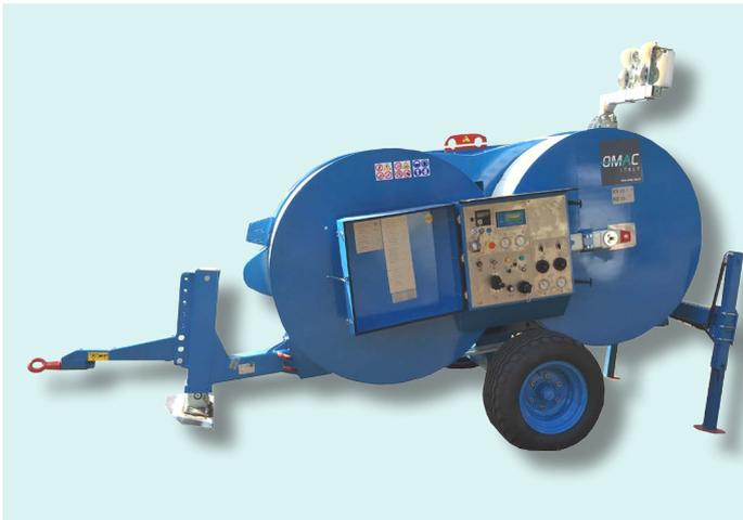
Hydraulic machine designed to operate both as a tensioner and as a puller, fit to string one rope or conductor. One hydraulic circuit allows to tension at constant force even varying the speed of stringing. In puller mode, one hydraulic circuit allows to continuously vary the speed in both directions.
