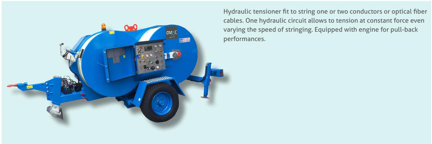
Hydraulic tensioner fit to string one or two conductors or optical fiber cables. One hydraulic circuit allows to tension at constant force even varying the speed of stringing. Equipped with engine for pull-back performances.
