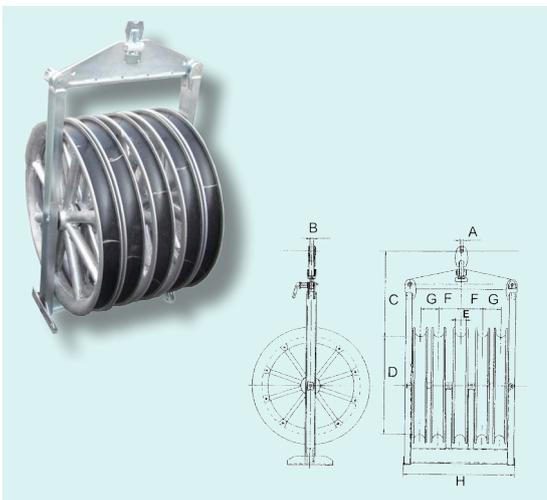
Five-sheave running out block fit for stringing four-bundled conductors. Aluminium sheaves mounted on sealed ball bearings. Grooves lined with nylon sectors. Galvanised steel frame with non-fleeting devices on lateral sheaves. Demountable attachment revolving by 90° (available with tight wheel).
