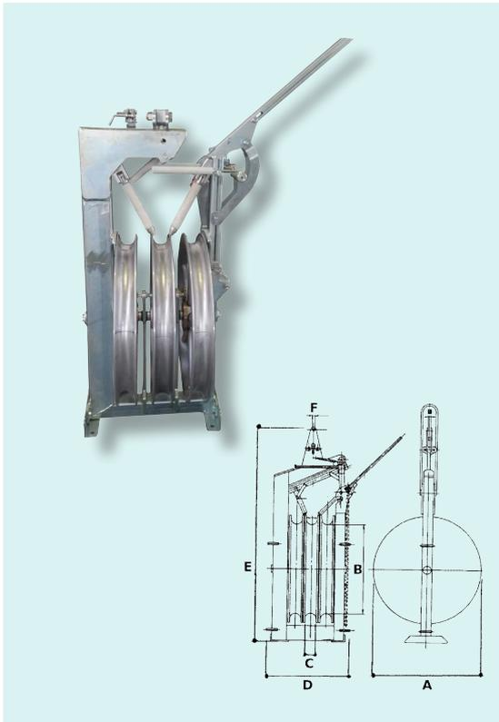
Three-sheave block fit for stringing a pilot rope by helicopter. Proper devices allow to position the pulling rope in the sheave groove, and keep it inside the groove during stringing operations. Aluminium sheave mounted on waterproof bearings. Groove lined with nylon sectors. Galvanized steel frame. Fix attachment.
