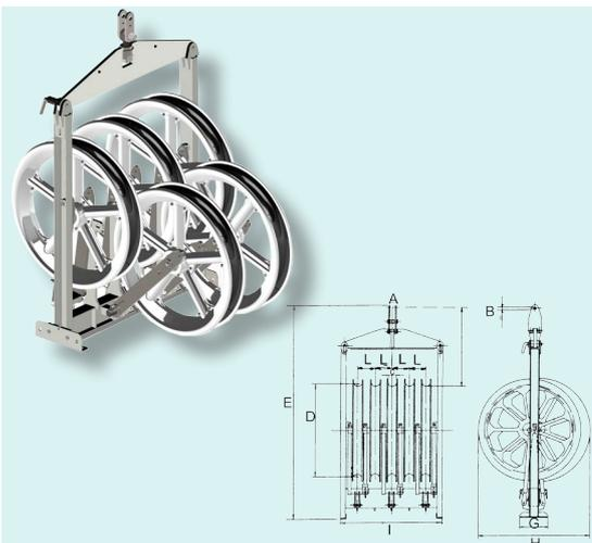
Detachable five-sheave running out block fit for stringing four-bundled conductors. The frame contains 5 running-out blocks that can be used singularly. Aluminium sheaves mounted on sealed ball bearings. Grooves lined with nylon sectors. Galvanised steel frame. Central sheave mounted on double bearings. Demountable attachment revolving by 90°.
