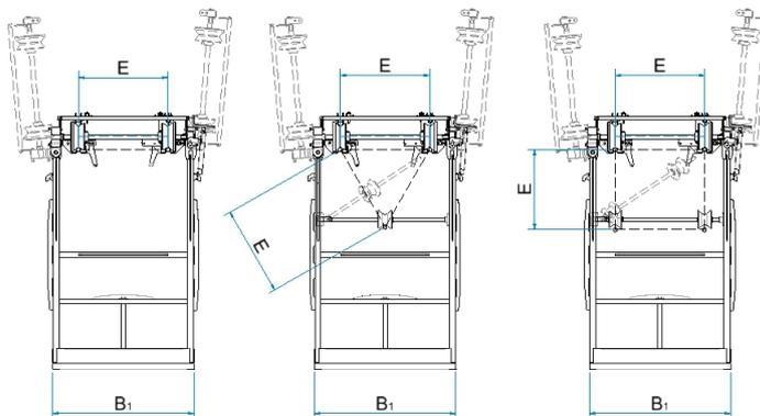
note:the dimensions E are adjustable 400-457-500-600 mm. Line cars with different dimensions can be produced on request.
