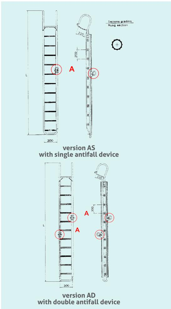
Ladder fit for vertical suspension, for working on transmission towers.
