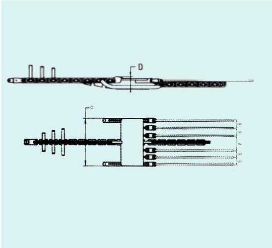
**Fixed type** running board for 6-bundle conductors fit for connecting the pulling rope to 6 conductors. The running board is made up of:
