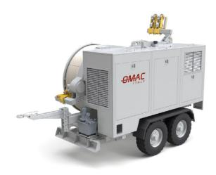
Hydraulic machine designed to operate both as a tensioner and as puller, fit to string one or two ropes or conductors. Two hydraulic circuits allow to tension at constant force even varying the speed of stringing. The two circuits can be used independently or simultaneously, with automatic forces partition. In puller mode, 2 closed hydraulic circuits allow to vary the speed in both directions, allowing to use one of the hydraulic circuits or both of them matched.
