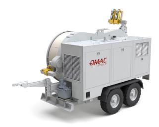
Hydraulic tensioner fit to string one or two conductors or fiber optic cables. One hydraulic circuit allows to tension at constant force even when the stringing speed changes.
