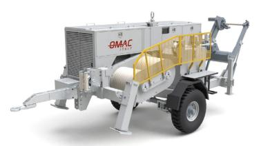
Hydraulic puller fit to pull one rope in overhead stringing operations. One hydraulic circuit allows to continuously vary the speed in both directions.
