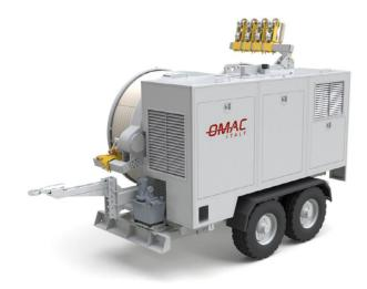
Hydraulic tensioner fit to string 1, 2, 3 or 4 (up to 6 on demand) conductors. One hydraulic circuit allows to tension at constant force even when stringing speed changes. Equipped with engine for pull-back performances.
