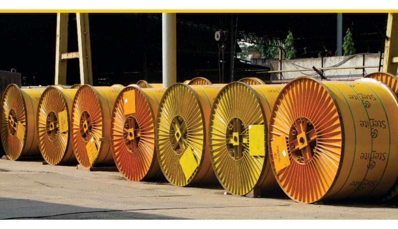
The packing of the conductor is an integral part of the manufacturing process, and the kind of package must be predetermined before production can begin.
