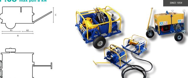
Hydraulic winch fit to pull one rope in service operations and laying underground cables. The winch can be disassemble into two parts. One closed hydraulic circuit allows to continuously vary the speed in both directions by operating one control device.
