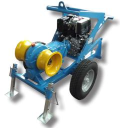
Mechanical winch fit to pull one rope while laying underground cables. The motion to the capstans is transmitted through a multiple-disk clutch and a gearbox, operated by means of 2 levers.
