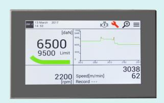
Electronic instrument for monitoring the working values.
