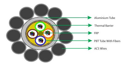
This design is suitable for high fiber counts under high heat dissipation requirements. The cable is ideal for lower span lengths & distribution transmission lines
