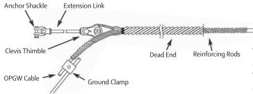
Tension Assemblies are designed for use with OPGW cable at termination, section and joint tower positions. They will hold upto 95% of the OPGW RTS and maintain optical integrity over the operating load range.
