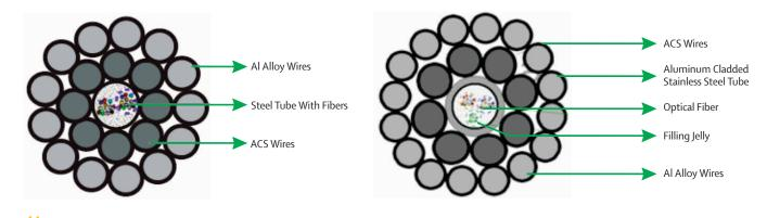
Ideal design for transmission lines with very high fault-current requirement
