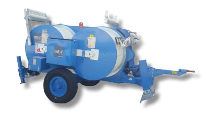
Hydraulic tensioner fit to string 1, 2 or 3 conductors. One hydraulic circuit allows to tension at constant force even varying the speed of stringing. Equipped with engine for pull-back performances.
