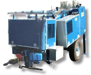
Hydraulic tensioner fit to string 1, 2 or 3 conductors. Three hydraulic circuits allow to tension at constant force even varying the speed of stringing. The three circuits can be used independently or simultaneously, with automatic forces partition. Equipped with an engine for pull-back performances. In pull-back mode, three hydraulic circuit allow to vary the speed in both directions, allowing to use one of the hydraulic circuits or all of them matched.
