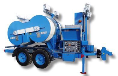
Hydraulic tensioner fit to string 1, 2, 3 or 4 (up to 6 on demand) conductors. Two hydraulic circuits allow to tension at constant force even varying the speed of stringing. The two circuits can be used independently or simultaneously, with with automatic forces partition. Equipped with engine for pull-back performances. In pull-back mode, two hydraulic circuit allow to vary the speed in both directions, allowing to use one of the hydraulic circuits or both of them matched
