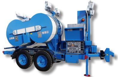
Hydraulic tensioner fit to string 1, 2, 3 or 4 conductors. Two hydraulic circuits allow to tension at constant force even varying the speed of stringing. The two circuits can be used independently or simultaneously, with automatic forces partition. Equipped with engine for pull-back performances. In pull-back mode, two hydraulic circuit allow to vary the speed in both directions, allowing to use one of the hydraulic circuits or both them matched.
