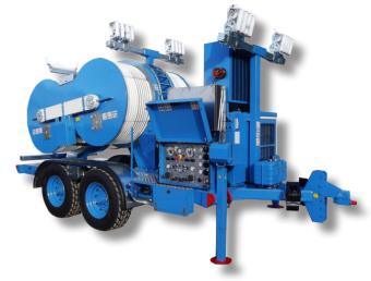
Hydraulic tensioner fit to string 1, 2, 3 or 4 conductors. Four hydraulic circuits allow to tension at constant force even varying the speed of stringing. The 4 circuits can be used independently or simultaneously, with automatic forces partition. Equipped with engine for pull-back performances. In pull-back mode, four hydraulic circuit allow to vary the speed in both directions, allowing to use one of the hydraulic circuits or all of them matched.
