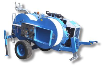
Hydraulic tensioner fit to string one or two conductors. Two hydraulic circuits allow to tension at constant force even varying the speed of stringing. The two circuits can be used independently or simultaneously, with automatic forces partition. Equipped with engine for pull-back performances. In pull-back mode, two hydraulic circuit allow to continuously vary the speed in both directions, allowing to use one of the hydraulic circuits or both of them matched.
