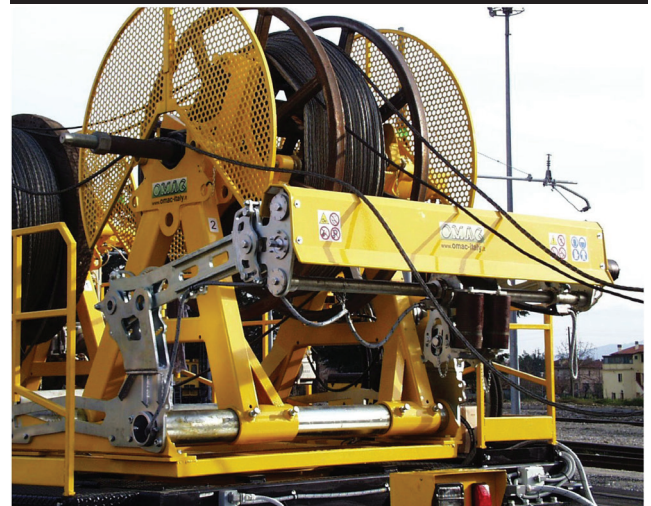
Automatic Wire/Cable Winder on the Last Reel-Stand (opt. 439)
