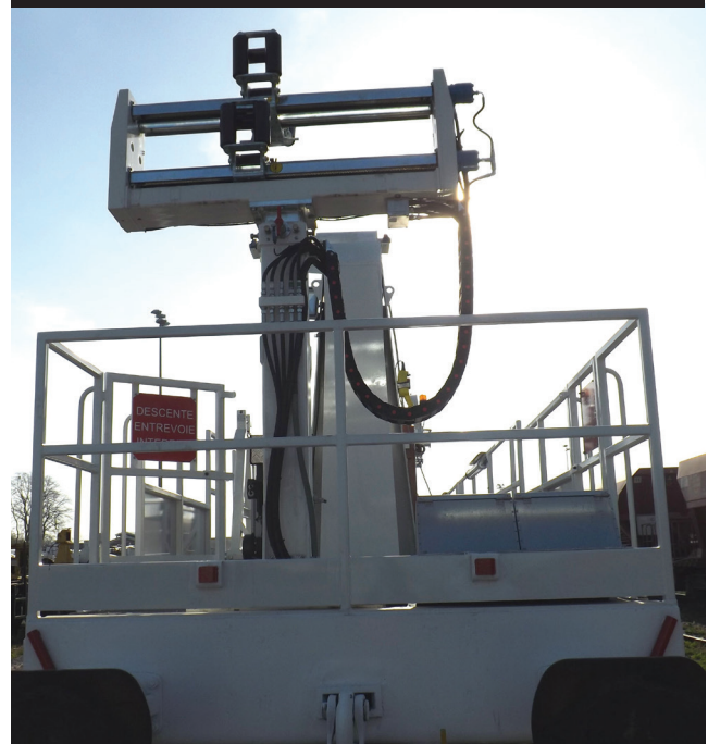
Automatic Wire/Cable Winders, Mounted on the Mast (opt. 445.2)
