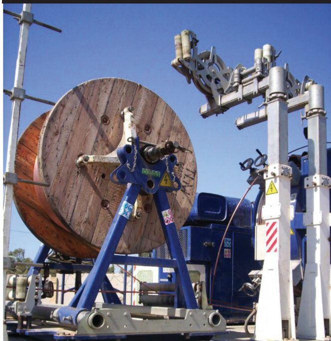
Device to rotate the Reel-Stand by \pm 90^\circ (opt. 419.2)
